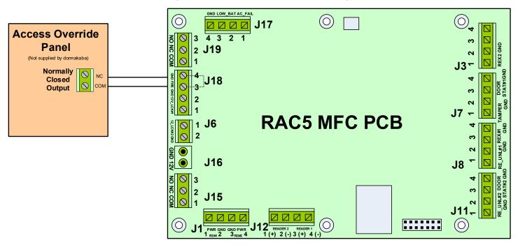
**Note 1:** The input from the Access Override Panel must be connected to a Normally Closed Dry contact. When the RAC5 MFC Access Override is activated, power to all relays will be removed. Ensure you have configured Switch 4 of the Relay Expansion Board appropriately for your desired controller behavior. See Switch 4 configuration details referenced on page 12.
