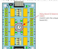
Each REB is factory configured to have a unique ID. If service to a REB is ever required, ensure to set the switch to the same ID of the PCB you are replacing.
